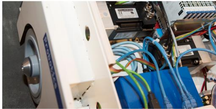
Optec uses synchronous servomotors from the KOLLMORGEN AKM range in a 48 volt version as drives for both wheels
