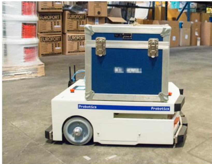
The AIVs weighing 40 kilograms can transport useful loads of up to 150 kilos
